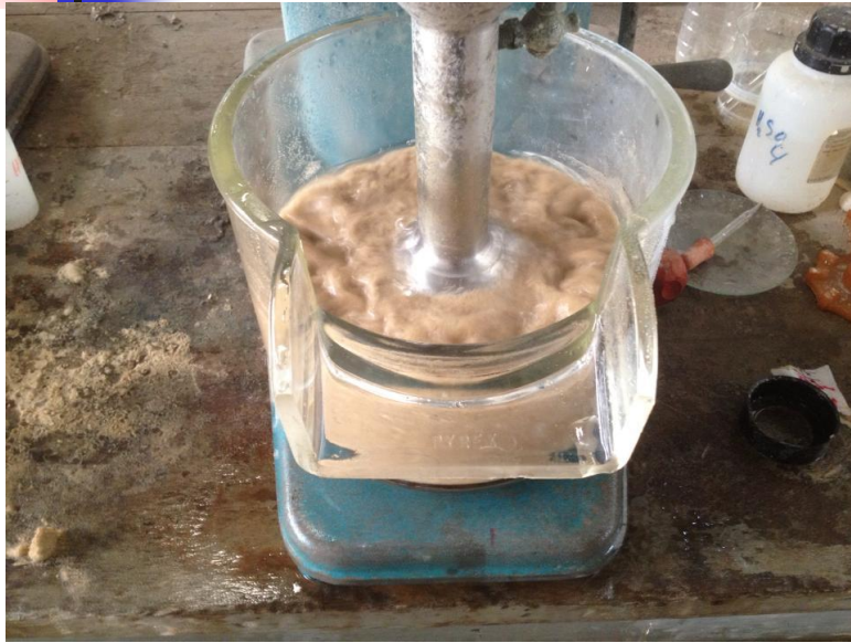
Scrubber to reduce \text{Al}_2\text{O}_3
