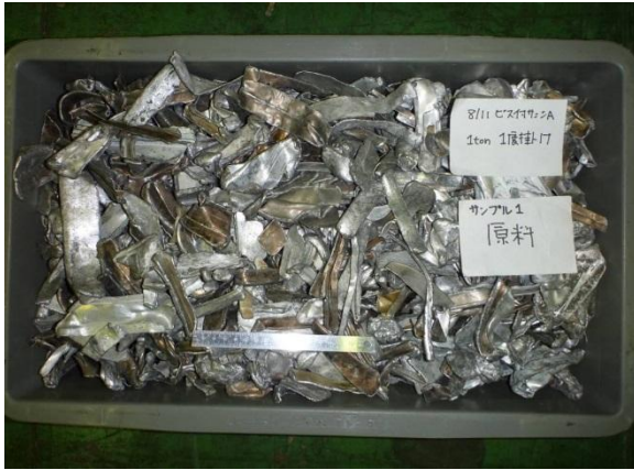
Real scrap sash shredded in a recycler left: Sample A, center: Sample B, right: Sample C, 800 kg each
