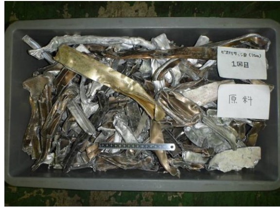
Real scrap sash shredded in a recycler left: Sample A, center: Sample B, right: Sample C, 800 kg each
