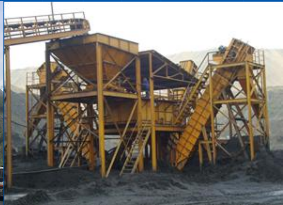
Fig. 3 Snapshot of an industrial moving screen jig erected at Ha Tu coal mine
