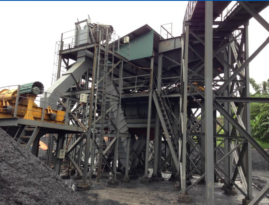
Fig. 5 Snapshot of an industrial moving screen jig working at Tan Lap mine
