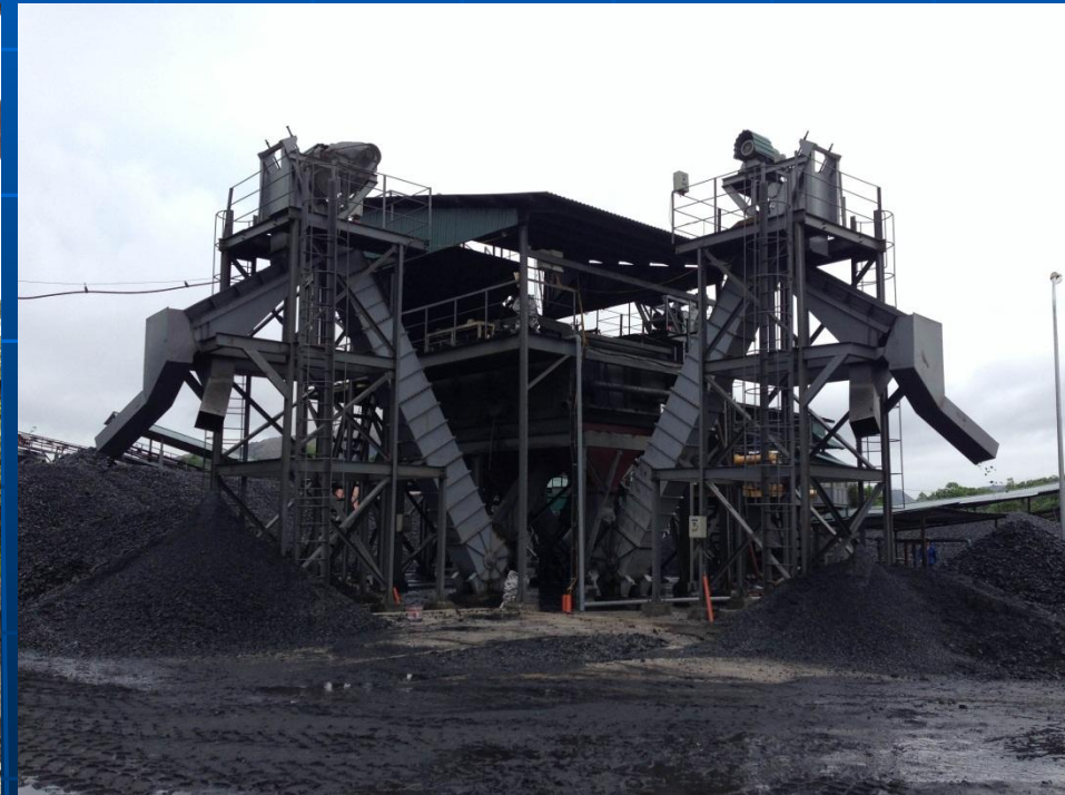
Fig. 5 Snapshot of an industrial moving screen jig working at Tan Lap mine
