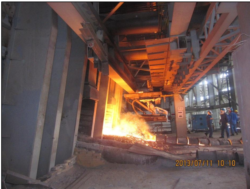
Fe-Ni molten metal tapping
