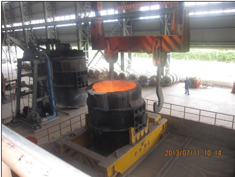
Crude Fe-Ni sent to refining stage
