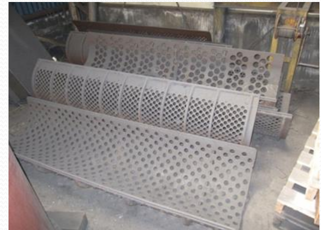
Screen for single-shaft crusher ( \Phi 200 mm)
