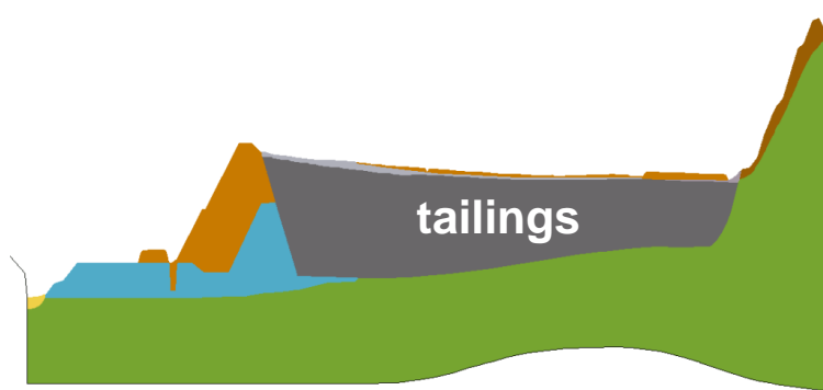
Cross sectional view of tailings dam
