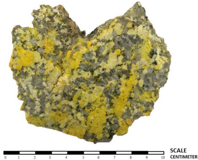
Figure 1 Stained hand specimen of monzogranite (CR 007 RK), dark yellow = alkali feldspar, light yellow = plagioclase, color less = quartz, dark mineral = biotite.
