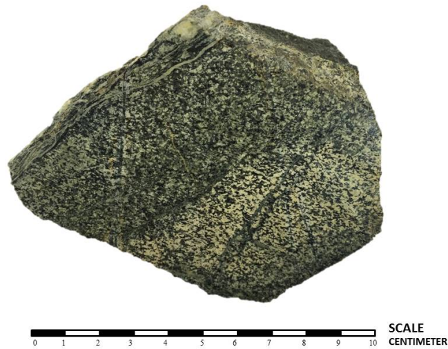
Figure 1 Stained hand specimen of cumulus gabbro (CR 024), white = plagioclase, dark = mafic minerals (pyroxene, unidentified mafic minerals and hornblende) and opaque mineral.
