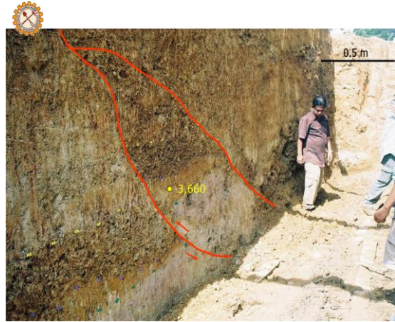
Trench of the sediment in undulating terrain along the Khlong Marui Fault zone, Ban Bang Luak, Phang- nga-Surat Thani Provinces. The profile showing the movement of young quaternary sediments (red lines)
