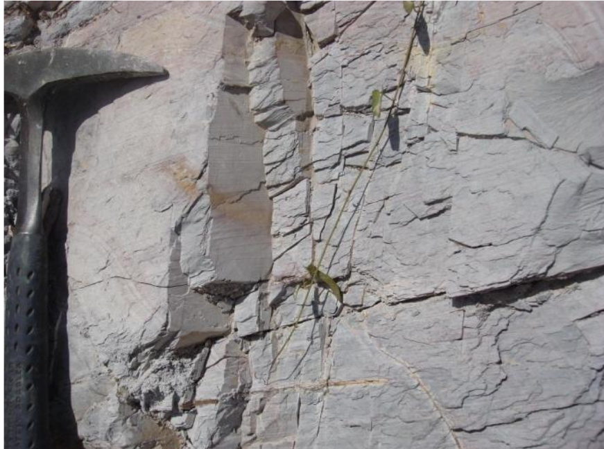
Figure 55: Closed-up of the laminated mudstone to claystone of the Middle mudstone and claystone member. (After The Malaysian-Thai Working Group, 2012)
